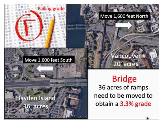
However, an immersed tube tunnel (ITT) requires only a 2,000-foot long grade at 3% from ground level to the center of the river. This allows an ITT to connect to the current on and off-ramps.
