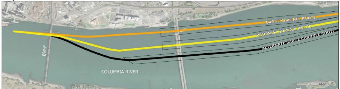
Figure 10. Existing and proposed channel routes within the Lower Columbia River federal navigation channel from Vancouver to Bonneville Lock and Dam; note proposed realignment and exchange of the relative location of the barge channel route (orange) and the primary channel route (yellow) (IBR, "Navigation Impact Report," rev. May 2022, 2-21).
