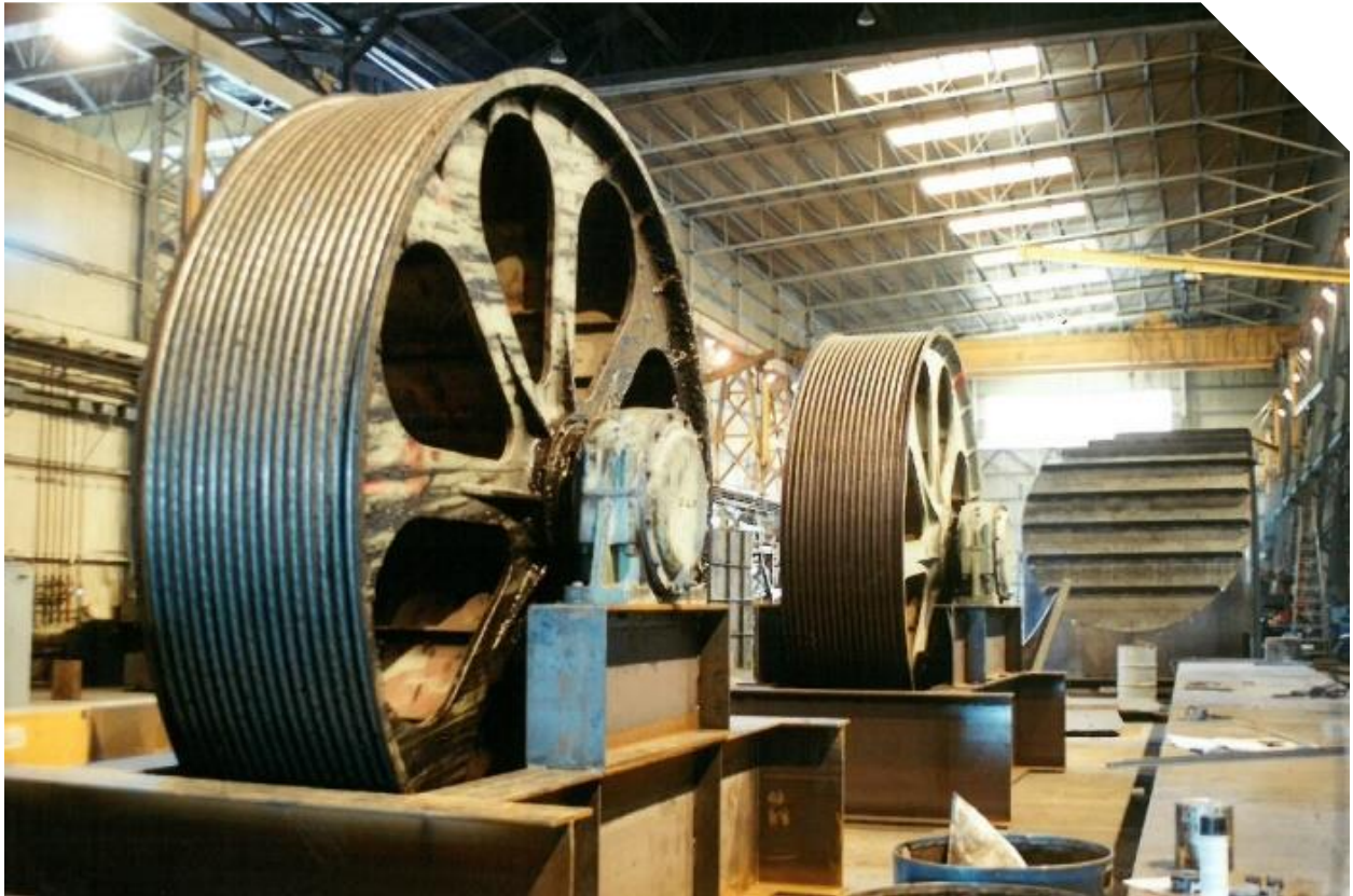
Trunnions for the Interstate Bridge shown above in Thompson's shop. Their proximity to the bridge made TMF an ideal location when repairs were needed. Shown below are two Seattle area bridge projects that were completed at the Columbia Business Center, painted by TMF, and delivered to the jobsite by barge.
