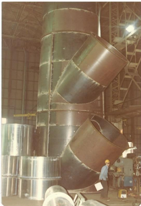
Heavy ducting for baghouses requires a facility like Thompson's. They can accommodate the size of the infrastructure in their shop and ship over the water by barge. The large duct section shown here is nearly 30' high and over 100' long.
