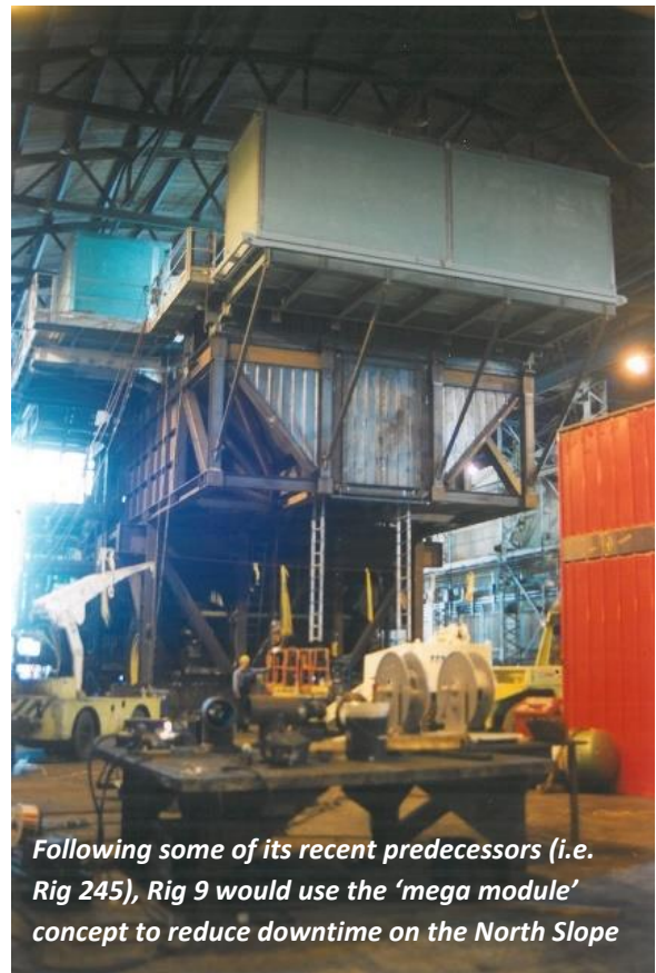
At 60' W x 30' H, this is one of many modules manufactured for Pool Arctic Rig 9
