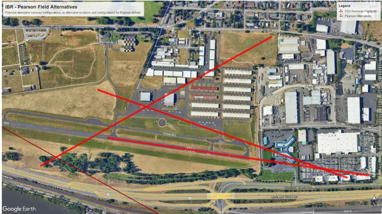
Photograph 2 – Some potential runway configurations and realignments at Pearson Field. Two options encroach into the parking lot of the Fred Meyer, but those businesses could easily be relocated to the part of the airfield which would not be needed. Basically, swap locations.
