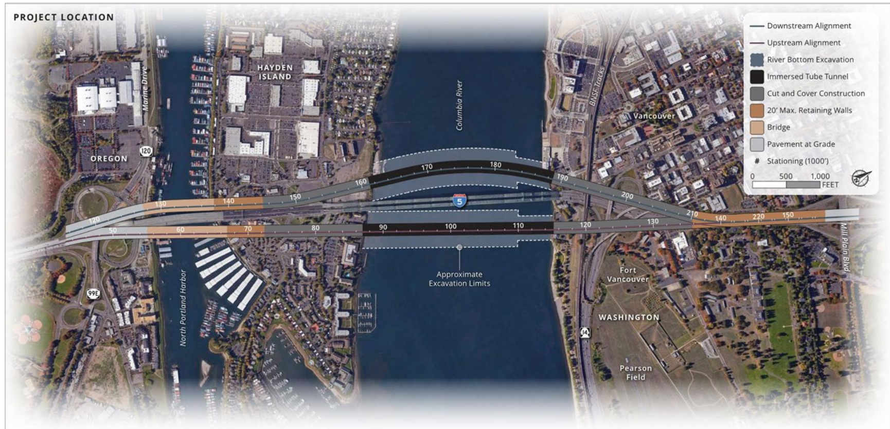
Figure 2. Upstream and Downstream Tunnel Alignments
