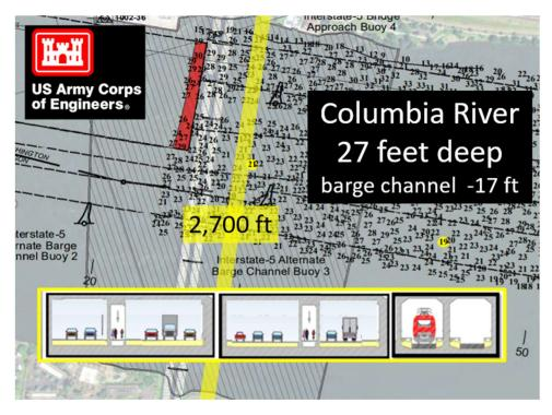
An immersed tunnel compared to a high bridge will annually save about 1.3 million gallons of carbon fuel and reduce green-house gases by 13 million tons. An immersed tunnel will be almost half as long and have half the total grade of a new high bridge. A high bridge has a long momentum killing uphill climb. A tunnel dip under the river adds momentum for a short climb. A shorter tunnel with less grade and downhill momentum, equals less total energy consumption, carbon or future kilowatt.
