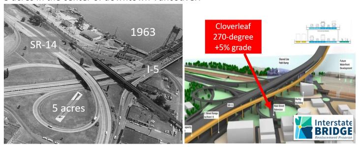
Cloverleaf 270-degree ramps are unsafe and are being replaced in New Jersey, Ohio, Texas, and California with 90-degree stacked ramps. An immersed tunnel comes up at ground level and offers an easy connection to a safer stacked ramp and a reduce ramp footprint.
