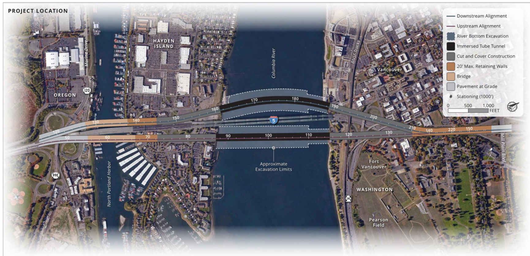
Figure 2. Upstream and Downstream Tunnel Alignments
