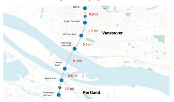
From 2015-2019, **55% of vehicle crashes within the Interstate Bridge program area were the result of rear-end collisions, and 19% were sideswipe crashes.** Auxiliary lanes are needed for substandard interchange spacing, lack of shoulders, and speed differential, not just stop and go traffic or congestion.
