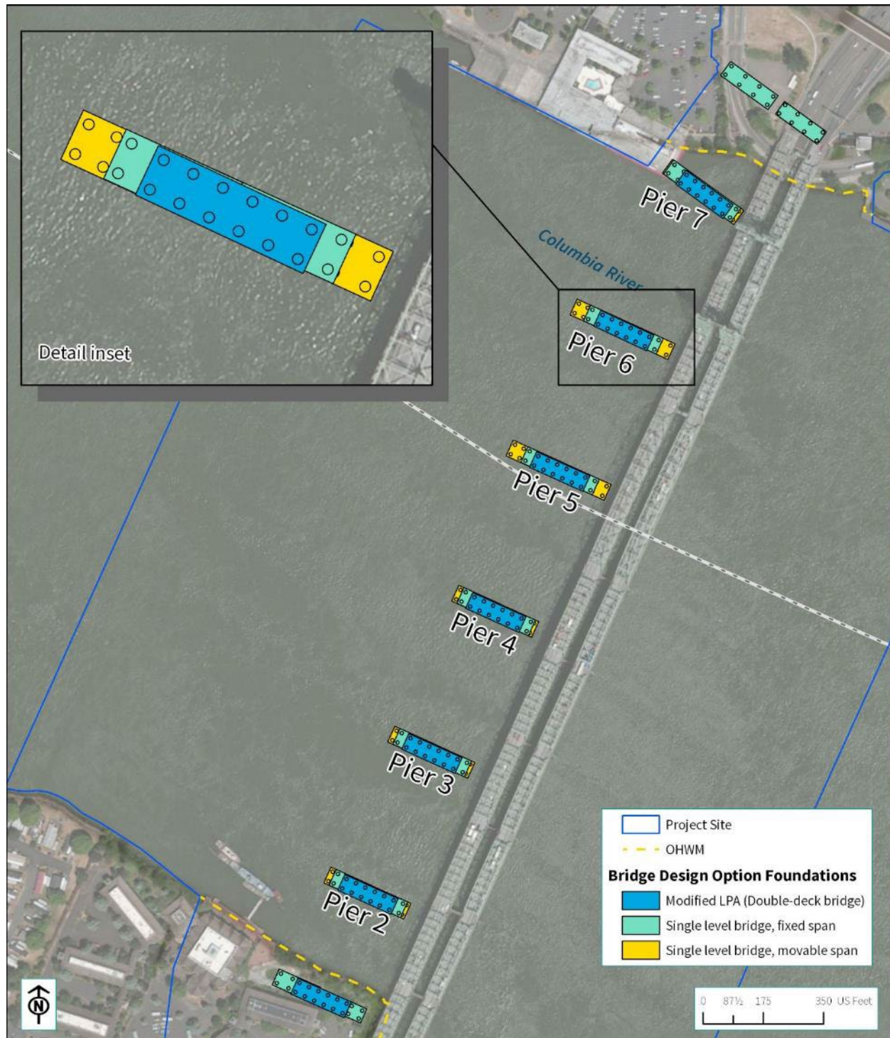
Figure 3-27. Columbia River Bridges – Design Option Foundations
