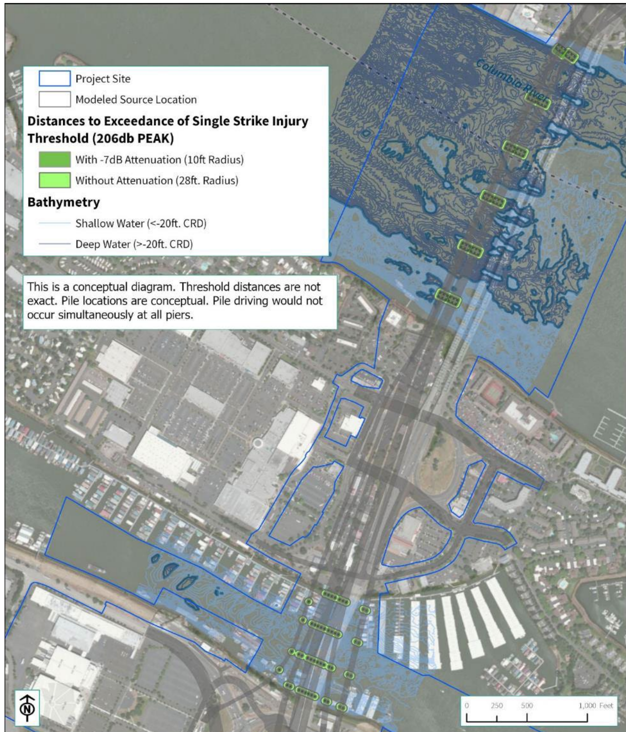
Figure 8-2. Distance to 206 dB Peak Injury Threshold for Fish during Impact Pile Driving – 18 to 24-inch Pile
