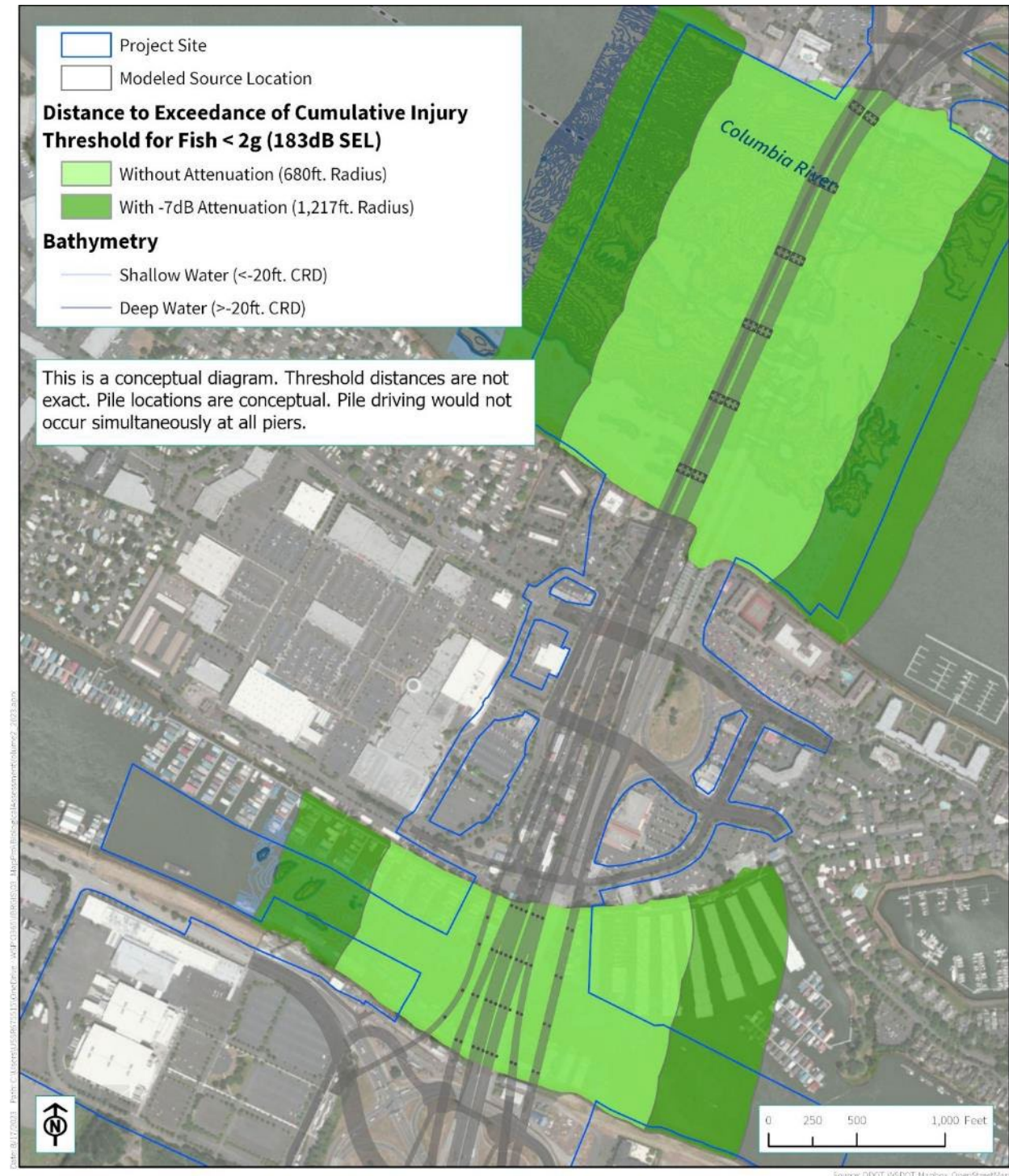
Figure 8-6. Distance to 183 dB SEL Cumulative Injury Threshold for Fish <2 g during Impact Pile Driving – 36 to 48-inch Pile, Single Pile Driver
