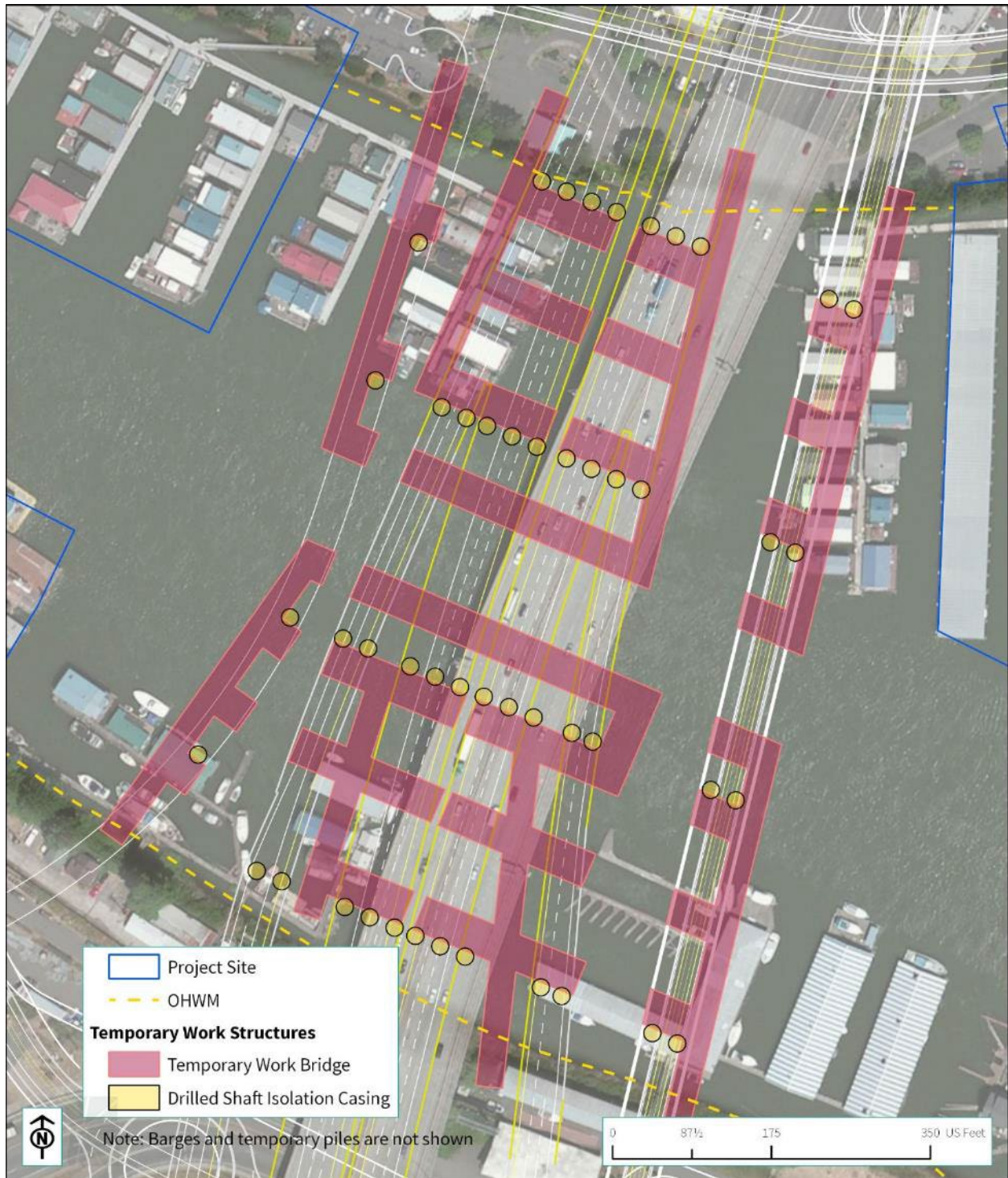
Figure 3-24. Temporary Work Structures – North Portland Harbor
