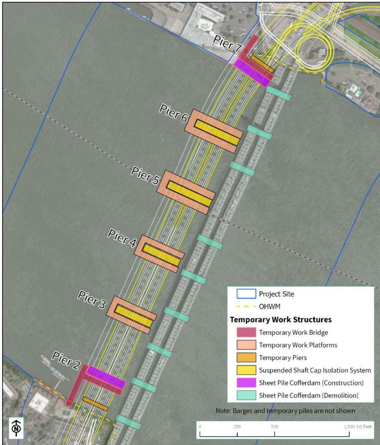
Figure 3-23. Temporary Work Structures – Columbia River
