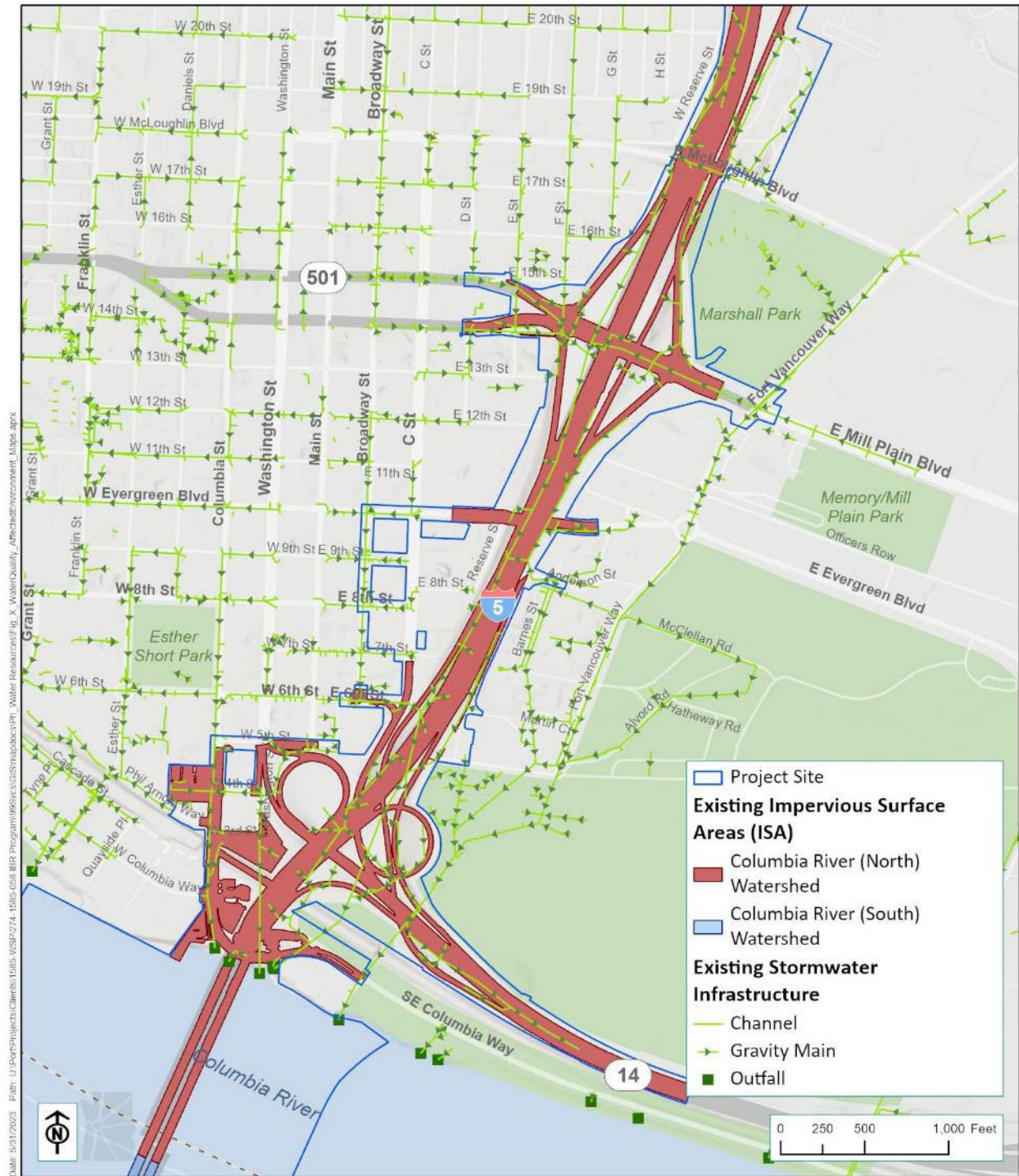
Figure 3-33. Stormwater Existing Conditions – Washington (South)
