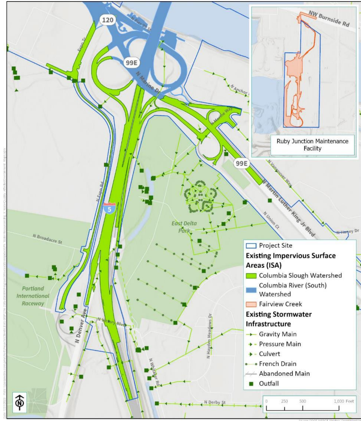
Figure 3-31. Stormwater Existing Conditions – Oregon (South)
