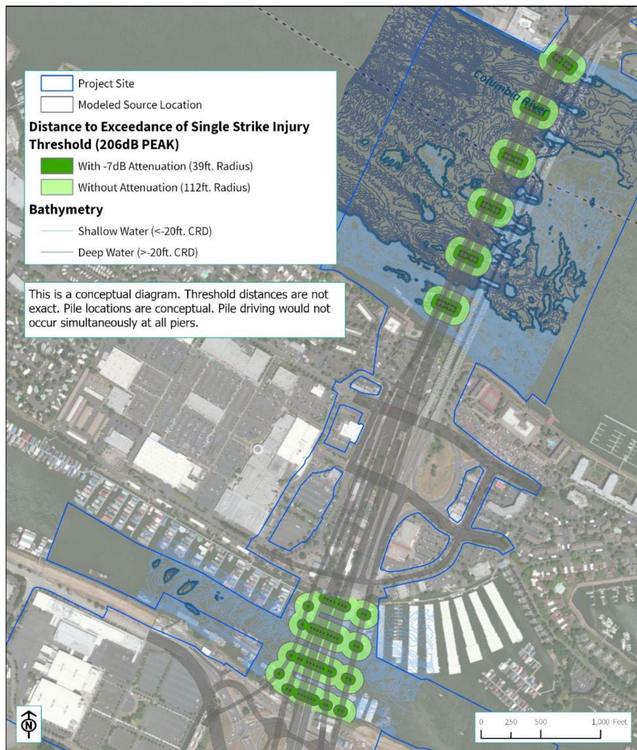
Figure 8-1. Distance to 206 dB Peak Injury Threshold for Fish during Impact Pile Driving – 36 to 48-inch Pile
