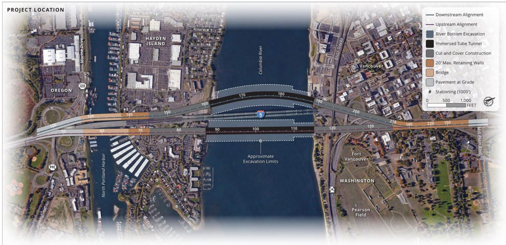
Figure 2. Upstream and Downstream Tunnel Alignments
